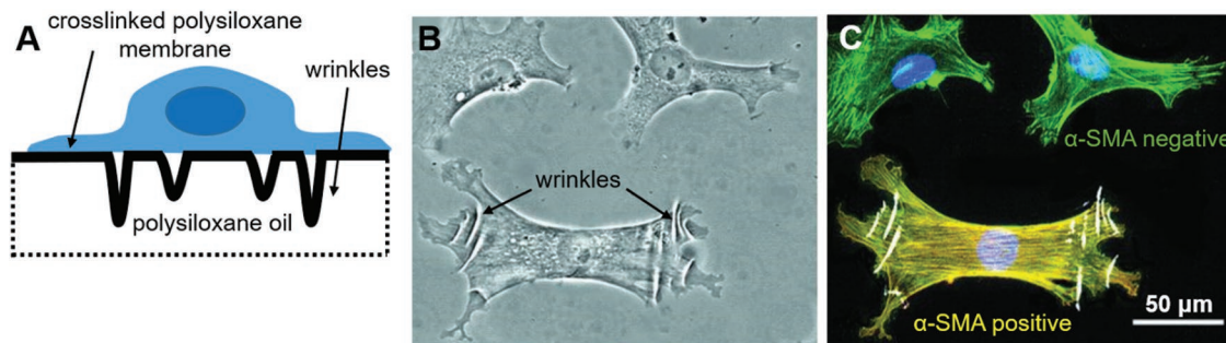
Figure 2. The first seminal method to study cellular forces involved polysiloxane wrinkling. A) Cells were seeded on a polysiloxane fluid that was briefly exposed to a flame to crosslink a thin surface. Cellular forces deformed the membrane and caused it to buckle or wrinkle. B) Wrinkles in the polysiloxane membrane can be visualized under light microscopy. C) When used in conjunction with fluorescent microscopy, the magnitude of cellular forces can be correlated with the expression of biomarkers. For example, a fibroblast that is positive for \alpha -smooth muscle actin (SMA) (yellow) create cellular forces that produce visible wrinkles, unlike those that are negative for \alpha -SMA (green). (B,C) Adapted under the terms of the Creative Commons Attribution 3.0 Unported. [14] Copyright 2001, the Authors. Published by The American Society for Cell Biology.
